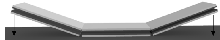
Picture 3.7: Principle of controlled rotational mounting of the magnet yokes
