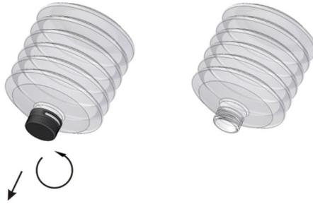
7. Place the cartridge on the inlet, install the prepared transparent cover
