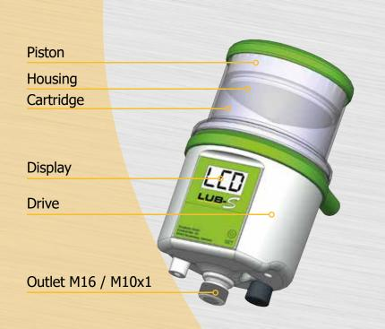
Two types of **Lubricus S** are available: **LUB-S-B** runs with a **4.5 V battery** and operates at 15 or 35 bar (218 or 508 psi). **LUB-S-V** uses **24 VDC** and can be connected to PLC optionally.
