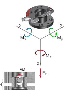
This guideline applies to the following assumptions: Acceleration: 10 m/s<sup>2</sup>, gravity distance: 100 mm, double safety
