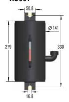
Oil capacity 2600 cm<sup>3</sup> Material: Steel
