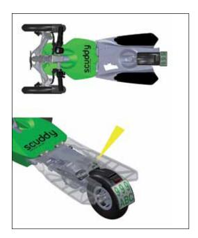
Compact, maintenance free, comfortable and also suitable for a load capacity of 100 kg: the tandem construction with TR52-32H type TUBUS profile dampers, which absorb up to 11.7 Nm/Cycle.
