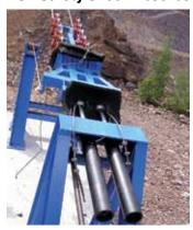
ACE safety shock absorbers are designed for emergency-stop situations in industrial and crane applications. They are individually tailored to the relevant application for emergency-stop.
