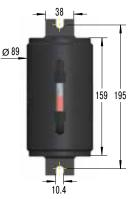
Oil capacity 370 cm<sup>3</sup> Material: Steel
