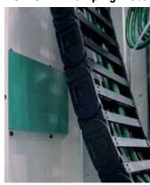
ACE-SLAB damping plates work using the visco-elastic damping of impacts and oscillation and offer constructors new perspectives for the large-scale energy absorption or customer-specific forms. Thanks to the simple installation using adhesives, they are an ideal solution for many damping requirements, for noise reduction and for the absorption of vibrations.
