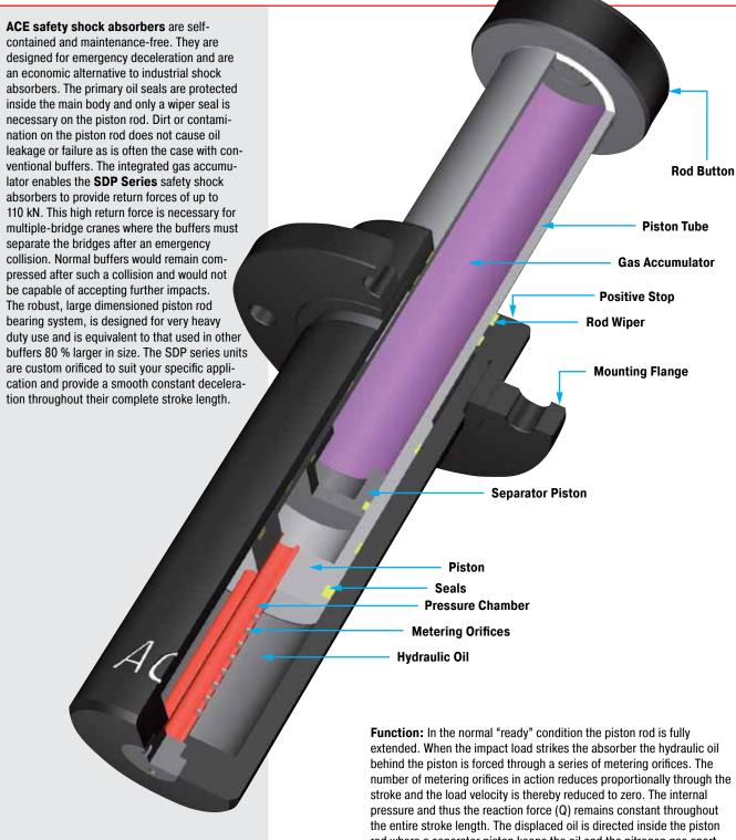
rod where a separator piston keeps the oil and the nitrogen gas apart. The integrated gas accumulator, containing low pressure nitrogen, provides the high return force to reset the rod to its extended position
