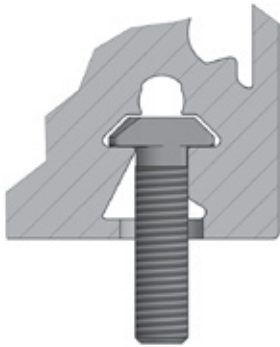
Figure 6.7 ___ Linear Axis AXF with hammer screws
