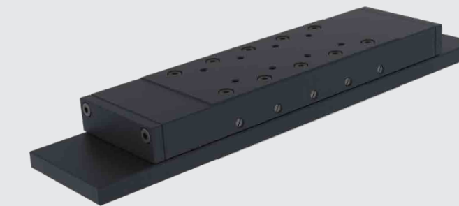
A crossed roller slide type RTNG offers protection against environmental contamination due to its narrow gap between table and base. Stroke range from 10 – 250 mm with a maximum load rating of 35.100 N.
