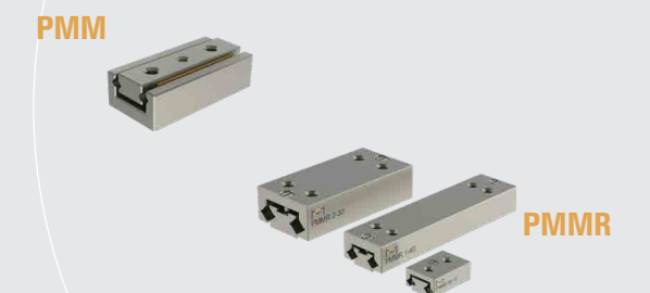
Micro slides of type PMM and PMMR are available with stroke lengths ranging from 5 to 70 mm in 3 different sizes. The weight specifications range from 2 to 80 grams. PMMR uses a crossed roller configuration for high stiffness and increased lifetime, intended for rapid and precise positioning in microscale applications.
