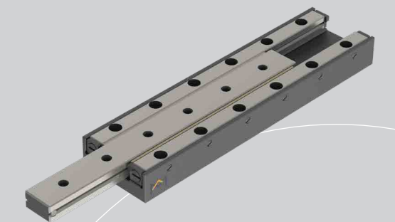
A low profile steel crossed roller slide RTS. Stroke range from 12 – 130 mm with a maximum load rating of 3.672 N.
