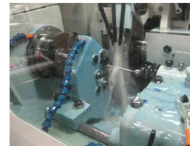
High accurate shaft groove process by Grinding machine
