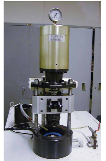
Photo B-11 : Pin-on Disk test machine
