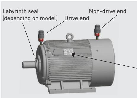
Lubrication points are located on the **drive** and **non-drive end of electric motors**. When relubricating, you must ensure that **excess grease is discharged** through the discharge openings, grease relief ports or grease traps. Bearings will overheat if grease cannot escape and / or if grease traps are filled up with used grease.
