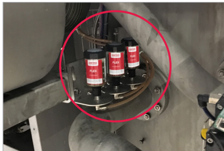
Remote pillow block lubrication on a belt weigher
