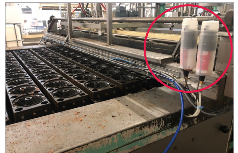
Oven chain lubrication on a baking line
