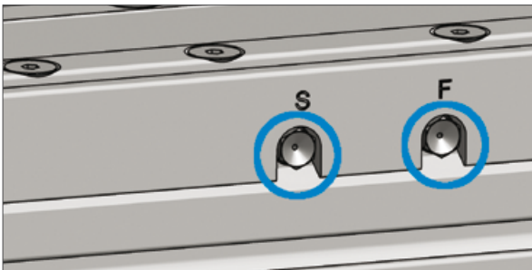
Figure 1.12 — Slider unit with laterally placed grease nipples
