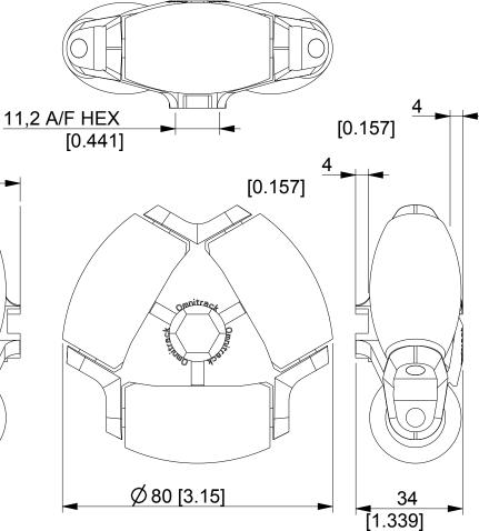
LOCK OMNIWHEELS TOGETHER IN SERIES FOR 360° SUPPORT
