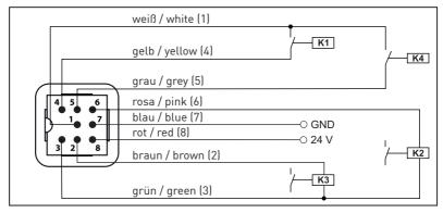
Fig. 10-3: Circuit diagram for connection via relays
