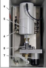
Fig. 3-2 Pump and distributor
