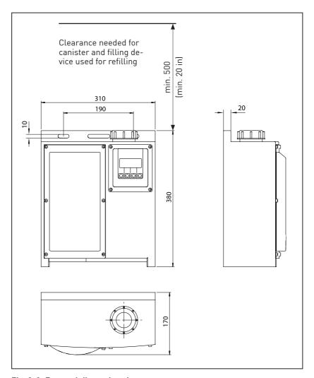
Fig. 3-3: External dimensions in mm
