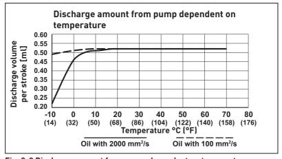
Fig. 9-2 Discharge amount from pump dependent on temperature
