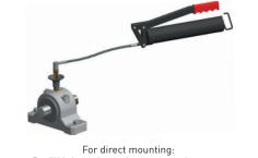
Prefill lube-point and any connecting parts (use the same grease that is contained in the lubrication system)
