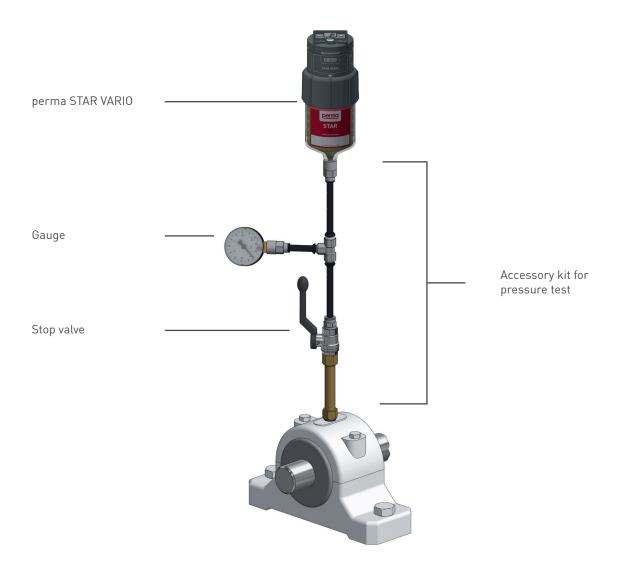
For pressure testing please use perma STAR VARIO with Accessory kit for pressure test (101480).
