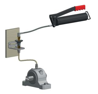
6. Use a tube prefill adapter to prefill lubrication point and grease lines.
