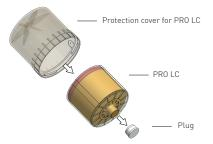
Place the PRO LC inside the protection cover and remove the plug of the PRO LC.
