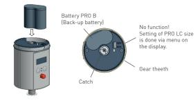
Insert the battery PRO B into the drive unit (according to the direction of the arrow on the label).
