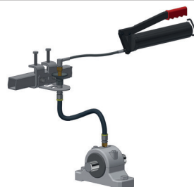
For remote mounting: Prefill lube-point and any grease lines / connections (use the same grease that is contained in the lubrication system)
