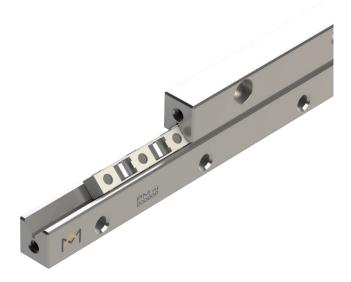
Our linear bearings type RSDE are a next generation development of the RSD type. The deeper V-groove in combination with uniquely designed cylindrical rollers and cages offer higher load ratings and stiffness without changing the boundary dimensions of the rails. RSDE rails are used mostly in highly dynamic applications requiring high speed, high running accuracy and outstanding quality.
