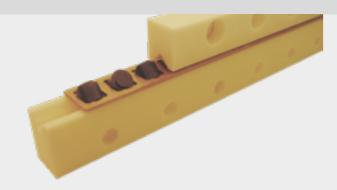
Fully ceramic linear bearing (CR) for applications requiring absence of magnetism, absence of lubrication or low mass combined with high stiffness. Commonly used materials are Si<sub>3</sub>N<sub>4</sub>, ZrO<sub>2</sub> or Al<sub>2</sub>O<sub>3</sub>. Typical fields of use include electron microscopy, semiconductor industry and medical applications.
