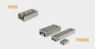
Micro slides of the <u>PMM</u> and <u>PMMR</u> types are available with stroke lengths ranging from 5 to 70 mm in three different sizes. Weight specifications range from 2 to 80 grams. <u>PMMR</u> uses a crossed roller configuration for high stiffness and extended lifetime, perfectly suitable for rapid and precise positioning in microscale applications.
