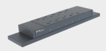
The <u>RTNG</u> crossed roller slide offers protection against environmental contamination due to its narrow gap between table and base. Available with stroke ranges of 10–250 mm and a maximum load rating of 35.100 N.
