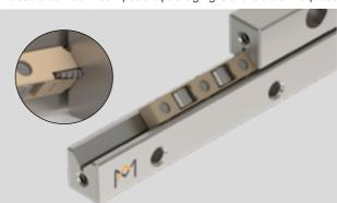
The standard crossed roller bearing with increased contact surface (RSDE or RNG) is equipped with cylindrical rollers and POM or PEEK cages and has a load rating three times that of standard RNG bearings. Available in roller diameter sizes 3, 4, 6 and 9 mm. Anti-cage creep technology (ACC) is available as an option.
