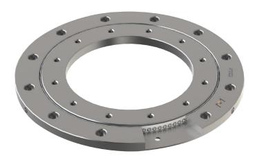
The precision Flat Mounted table Bearing (FMB) consists of two through hardened standard bearing steel rings and a teflon cage filled with steel balls precision-matched. The custom designed ball-groove increases load capacity and stiffness in moment loading while guaranteeing high precision, longer service life and a very low coefficient of friction. Pre-drilled attachment holes ensure easy installation.
