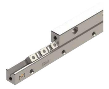
RNG linear bearings are compact, reliable and suitable for high loads. The RNG linear bearings in size 4 and 6 are a further development of the RSDE type, with more advanced mechanical characteristics. Significantly higher load ratings and stiffness are complemented by more compact installation dimensions, achieved through optimisation of the groove's internal geometry.
