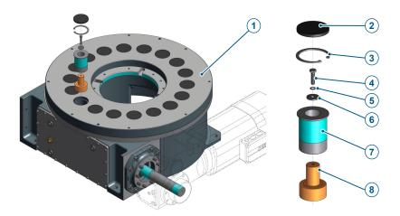
Fig. 16: Replacing the TMF2000 - TMF8000 cam follower
