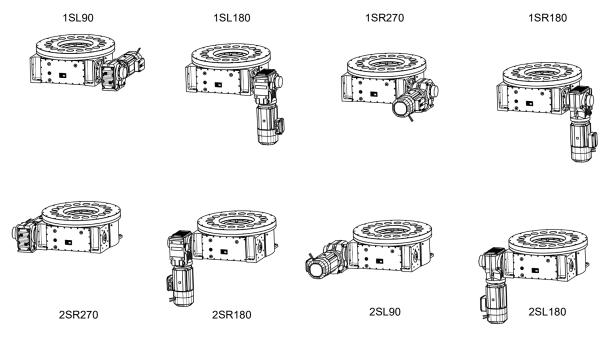
Fig. 8: TMF1000 – TMF5000 drive attachment positions
