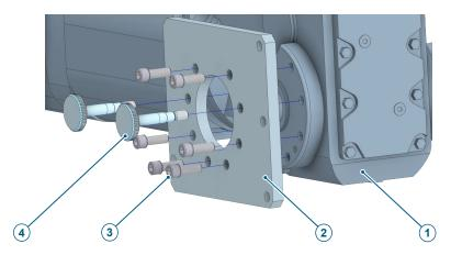
Fig. 11: Mounting the flange plate on the complete drive
