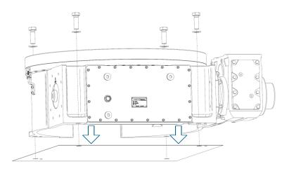
Fig. 14: Rotary indexer installation
