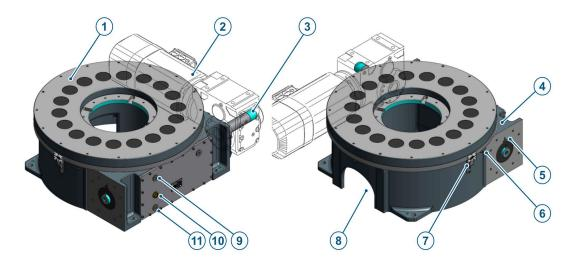
Fig. 4: Rotary indexer structure: TMF3000 - TMF5000
